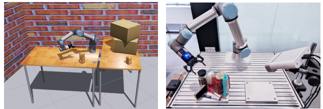
Figure 9. The IROS 2020 table organization challenge setup in simulator and the real world.
