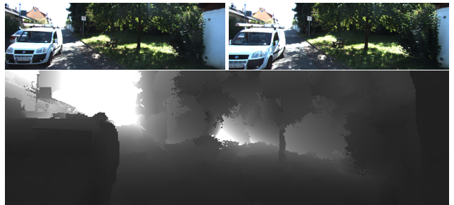
Figure 1: Given two frames from a monocular video of a dynamic scene captured by a single moving camera, our approach computes a dense depth map that reproduces the spatial layout of the scene, including the moving objects. Top: input frames. The white vehicle is approaching the camera, while the camera itself undergoes forward translation and in-plane rotation. Bottom: the estimated depth map.
