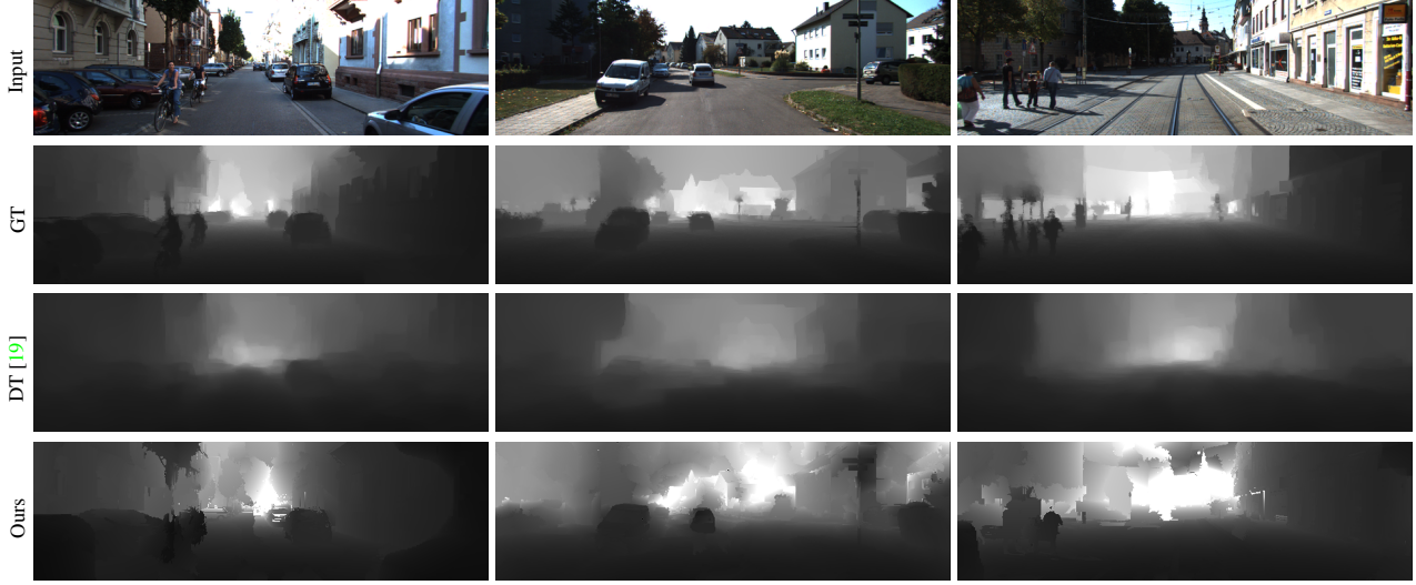
Figure 3: Results on three frames from the KITTI dataset. For each frame, the figure shows the input color image, the ground-truth depth (GT, inpainted for visualization), results produced by depth transfer (DT) [19], and results produced by our approach.
