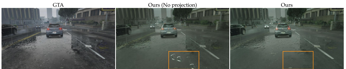
Fig. 19. Which discriminator?, continued. Adding the projection of semantic embeddings to the discriminator removes artifacts.
