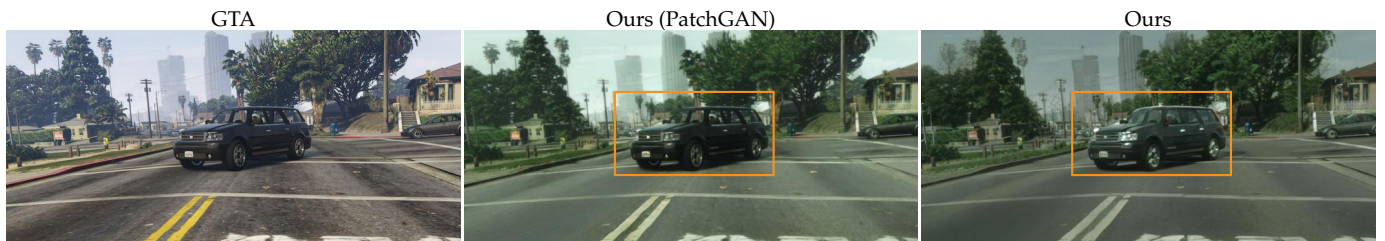
Fig. 18. Which discriminator? Our perceptual discriminator (right) is more effective than a PatchGAN discriminator (middle). Note the stronger enhancements such as lights and reflections on the car on the right.
