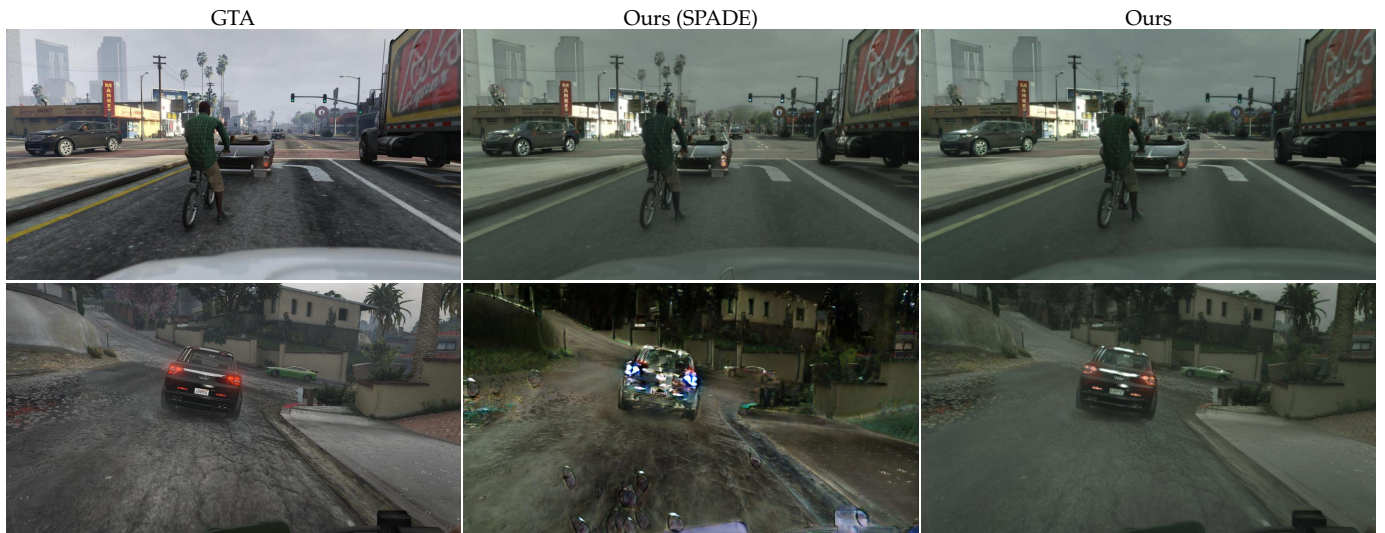
Fig. 17. How to ingest G-buffers? Enhancement of GTA images (left) using SPADE modules (middle) is highly volatile across the dataset (compare the top and bottom rows). Our RAD modules yield more consistent results (right).
