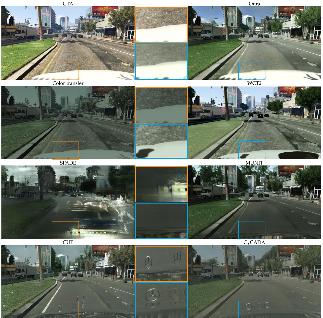
Fig. 14. We compare our results to original GTA images and a number of baselines. Our results are structurally consistent with the input. ColorTransfer does not modify textures. WCT2 strongly depends on a favorable reference image. SPADE fails due to differences in the scene layouts. MUNIT hallucinates trees, and CyCADA and CUT hallucinate star logos. Additional results for all baselines are shown in the supplement.
