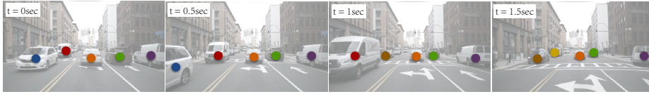
Fig. 1: We track objects by tracking their centers. We learn a 2D offset between two adjacent frames and associate them based on center distance.
